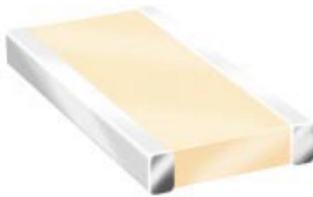
AVX's low inductance capacitors are designed for use in high speed circuits. Their aspect ratio and size have been optimized to reduce inductance from the 1 nH range found in normal chip capacitors to less than 0.4 nH. Their low profile is ideal for surface mounting or inside cavity mounting, adjacent to the IC itself.
